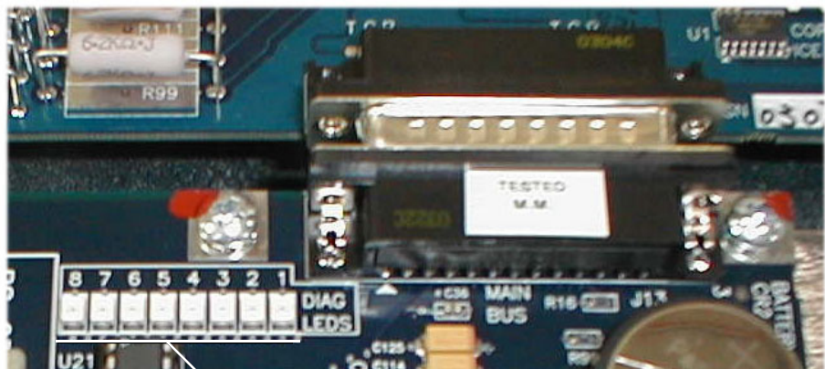
Figure 3.2 iLink CTP Board Diagnostic LEDs
