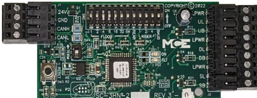
Figure 1.2 SC-3HN-2 Three Input Serial Hall Call Node Board, Gen. 2
