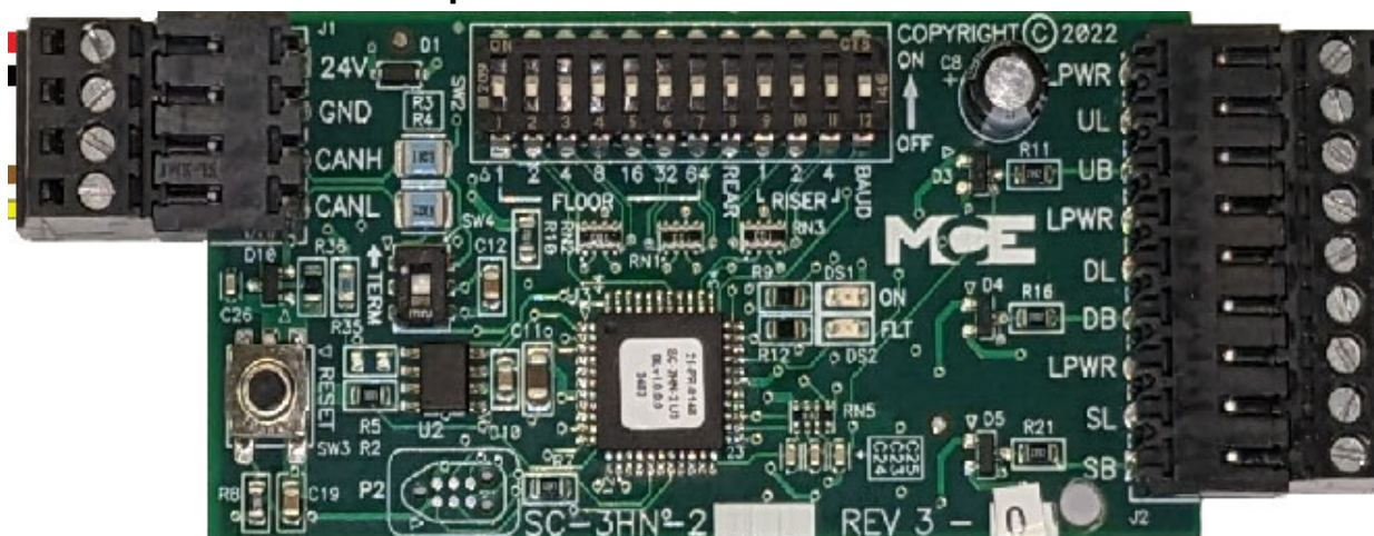
Figure 1.12 SC-3HN-2 Three Input Serial Hall Call Node Board. Gen. 2
