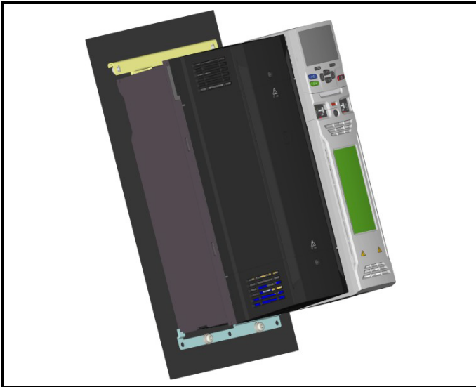
Figure 1-3 Locating the drive to the backplate
